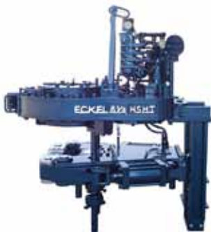
Eckel 8-5/8 HS HT Tong with Tri-Grip Backup
